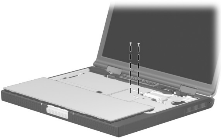
Figure C-7. Phillips M2.0 × 4.0 Screw Locations
